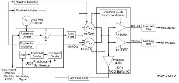
Figure 2. VHF/UHF Frequency Generation Unit (FGU) Circuits
