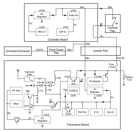
Figure 1A. DC Power Distribution Block Diagram (Closed Architecture Controller and VHF or UHF Transceiver)
