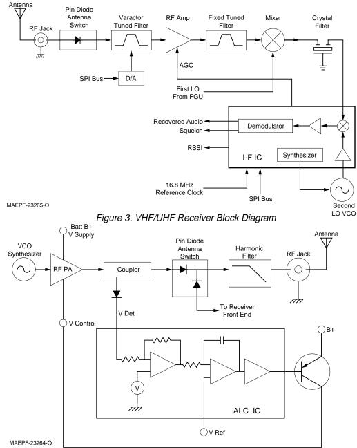
Figure 4. VHF/UHF Transmitter Block Diagram
