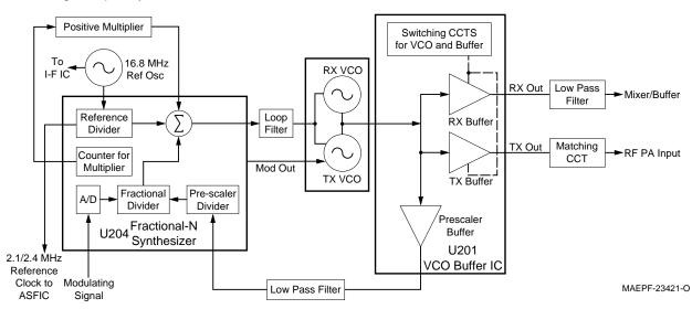
Figure 5. 800/900MHz Frequency Generation Unit (FGU) Circuits
