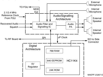
Figure 8. Closed Architecture Controller Block Diagram
