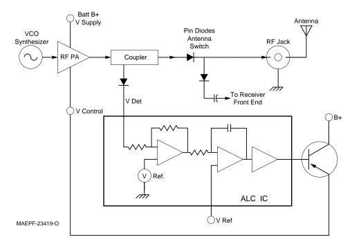
Figure 7. 800/900MHz Transmitter Block Diagram
