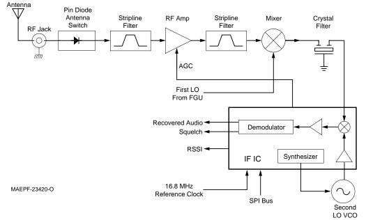
Figure 6. 800/900MHz Receiver Block Diagram
